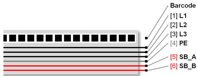
Fig. 2: Separate conductor lines [5] and [6]
