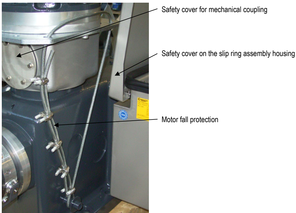
Figure 4.: Safety systems on the motor-driven reel
