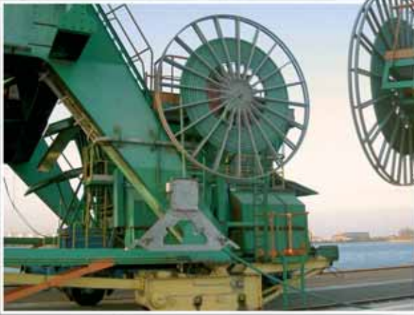
Motor driven reel with a monospiral spool and a two-way cable guide in action.
