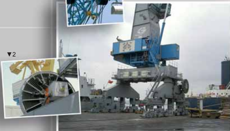
Mobile swiveling multi purpose crane power supplied with equipments of the MAG DRIVE reel range.
